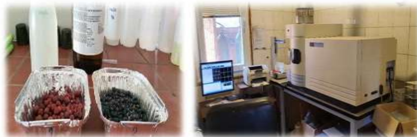
Figure 1. Collected samples and their analysis in Inductively Coupled Plasma; ICP-OES Perkin Elmer Optima 2100 DV, according to method EPA 6010C, 2007
