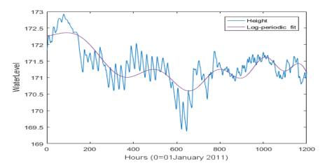
Figure 2. Time graph of water level in Koman, 01.01.2011-09.02.2011
