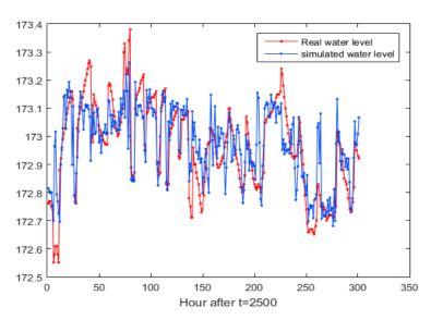
Figure 2. Prediction of the water level by changing the discharges from Fierza
