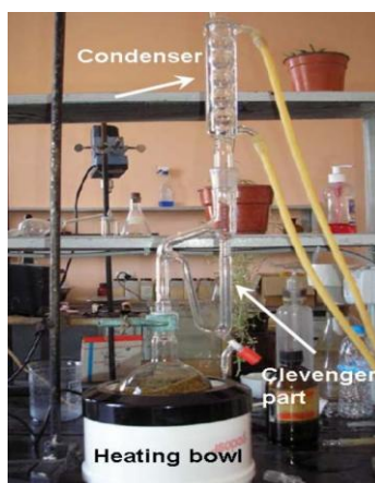
Figure 1: Photo of Clevenger apparatus used for the extraction with steam distillation indicating by arrows the main parts.
