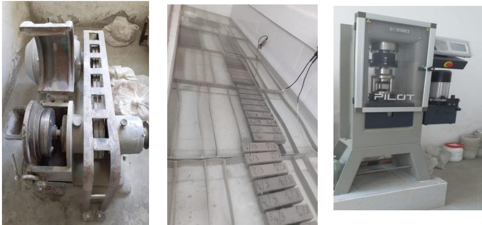
Figure 4. Laboratory mill with disks; bathtub where the prisms are kept; hydraulic press.
