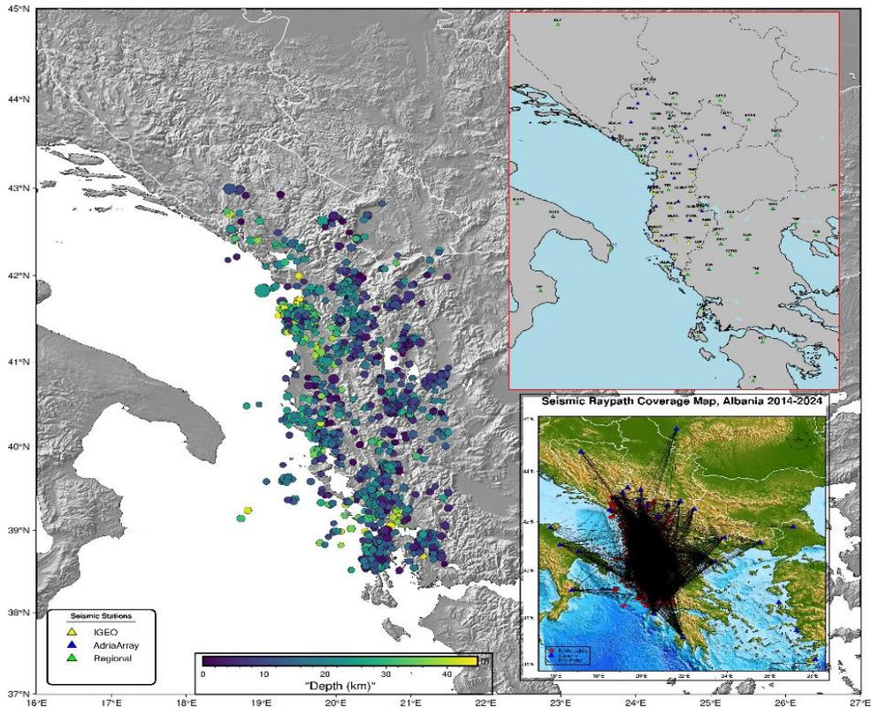
**Figure 3.** Spatial distribution of earthquake hypocenters in Albania and surrounding ( $M_L \geq 3.0$ ) recorded during the period 2014-2024; the seismic network used to record the data and the ray-path coverage map is also shown, on the map.
