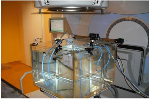
Figure 1: Setup geometry for PDD measurement and absolute dosimetry
