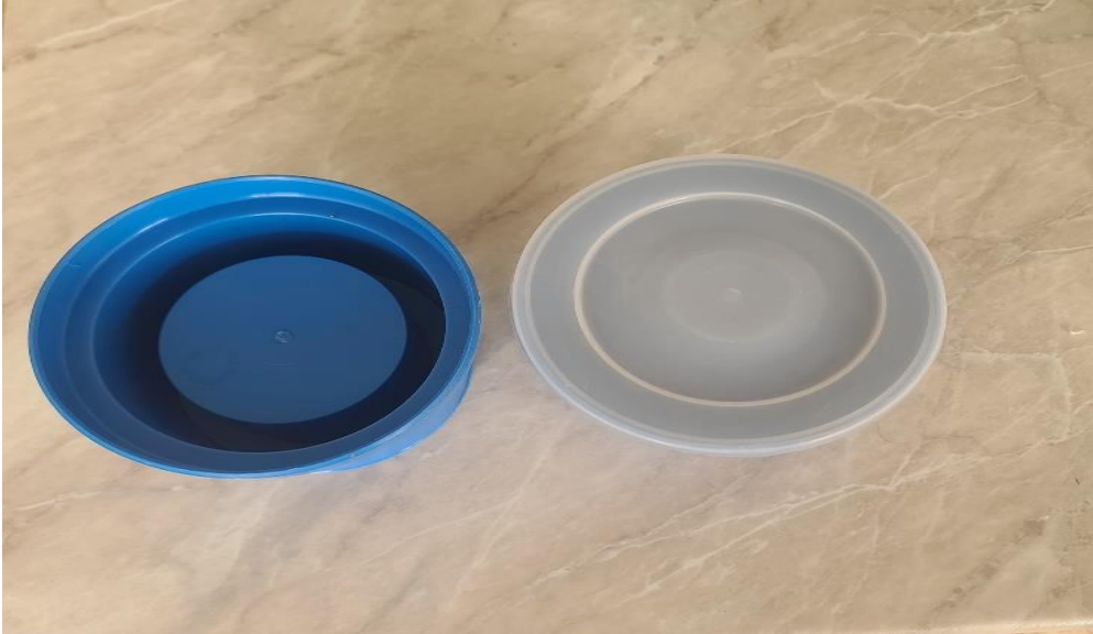
Figure 4, The Marinelli container used for gamma measurements. The container ensures consistent geometry for accurate determination of radionuclide concentrations in sample materials.
