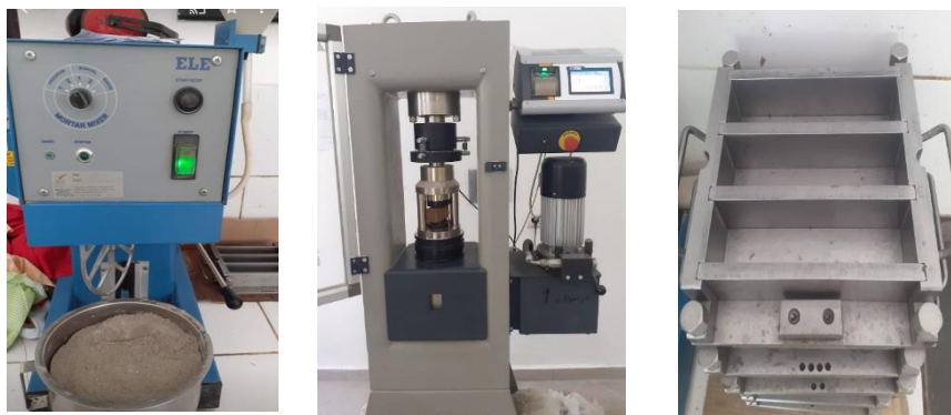
Figure 5. a). Mixer, b). Compressive strength machine, c). Prisms (40 mm x 40 mm x 160 mm).
