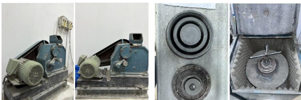
Figure 4. a). Jaw crusher PY 175 and, b). Ring mill GJ-100-1.
