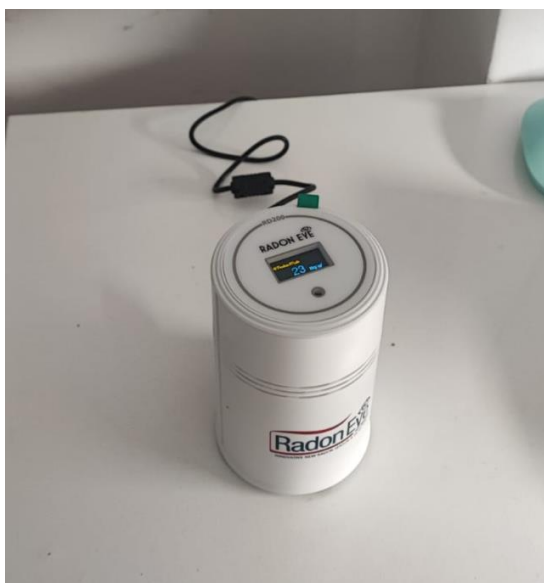
Figure 1. RadonEye RD200 radon detector deployed in situ in one of the monitored indoor environments during the measurement campaign.
